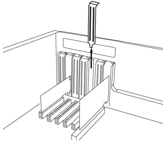
*Figure 4. Removing the PCI Slot faceplate*
