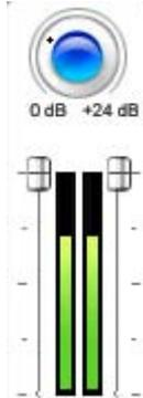
These are where you can adjust level for the analog input 1/2 and 3/4. The Input and Input monitoring levels can be set using the mouse, mouse wheel, or cursor keys.
