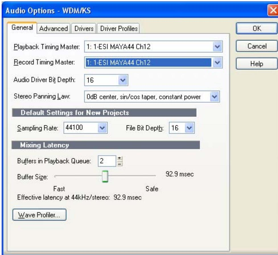
The input and output drivers have to be matched to each other. Restart the SONAR after the settings have changed.
