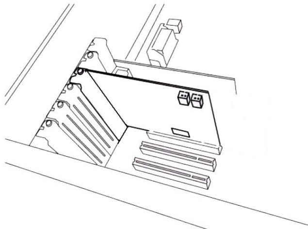
*Figure 5. MAYA44 Installed in a PCI slot*
