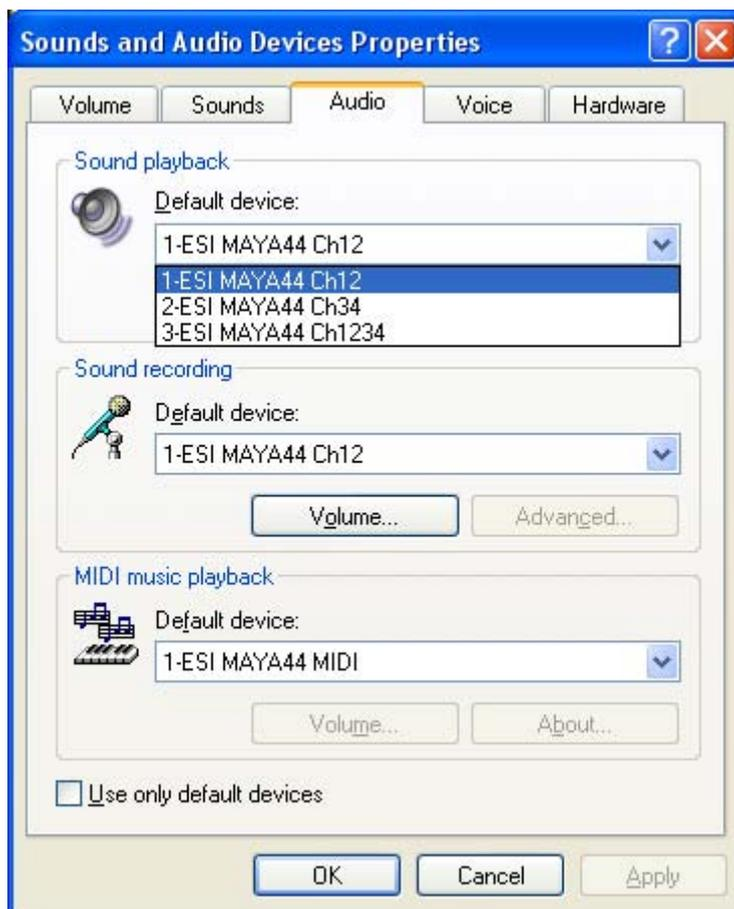
Some Advanced properties buttons will be grayed out because MAYA44 console panel has all input and output mixer controls which some of the mixer features are not compatible with Windows default mixer. However, this does not mean you do not have advanced options. MAYA44 console panel is designed to include all professional audio features that are not always compatible with the basic mixer control.
