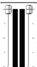
Display and change the level of the final output. The level can be set using the mouse, mouse, or cursor keys. Click the dB indicator to mute and un-mute the output.
