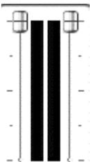
Display and change the output level for each source. The level can be set using the mouse, mouse wheel, or cursor keys. Click the dB indicator to mute and un-mute the output.
