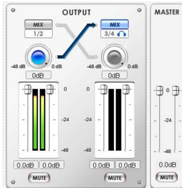
Adjusts and monitors the output levels of each audio channel via level faders and meters. You can also use output port 3/4 as a headphone jack. MAYA44 features a high-fidelity headphone amplifier.
