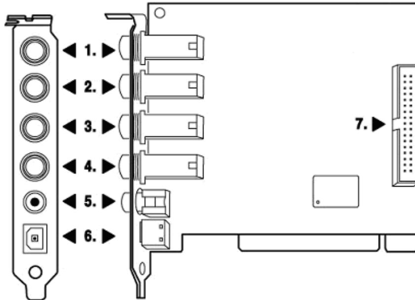
1. **LINE 1/2 Analog Input** Connector (Stereo Input) / MIC 1 Input (Mono Input)
