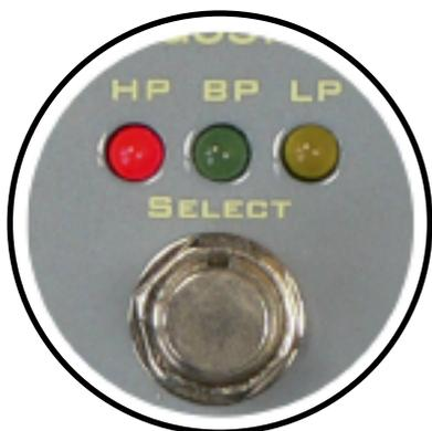
The Select switch offers three different presets....HP (high Pass), BP (Band Pass) and LP (Low Pass). These presets give you everything from the deepest growling 60's wah effect to the sharpest 70's disco sounds...and everything in between. With the Low Pass setting, the Classic Optical Envelope is also suitable to be used with bass guitar.
