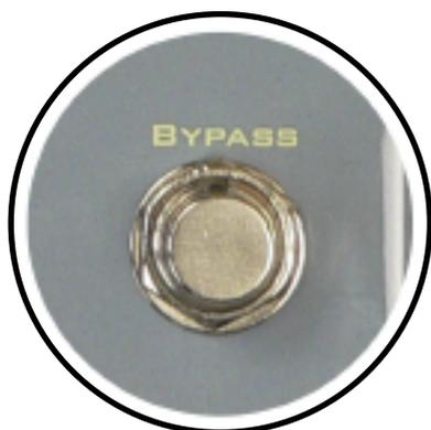
Our Bypass button on the Classic Optical Envelope simply switches the effect on and off. This is a high quality buffered bypass (NOT True Bypass) which ensures silent switching and no loss of high frequencies due to long cables or multiple pedals....a critical feature for envelope filters which rely on full bandwidth.
