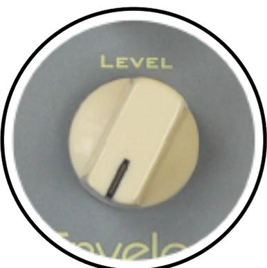
The Level knob adjusts the overall level of the Classic Optical Envelope. By adjusting this knob you can match or exceed the bypass signal.
