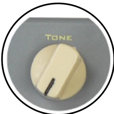
The Tone knob on the Classic Optical Envelope, is a high cut filter. With the knob set at full clockwise, you enjoy the full bandwidth of frequencies, so as you turn the knob counter clockwise, you start to filter out the high frequencies. On this effect, the Tone control works interactively with the Drive control, so as you adjust the Drive, you may find that you have to 'tweak' the Tone control to achieve your optimum tone.
