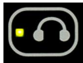
Normally, the headphones have their own D/A converter separate from the main outputs. This means that one track can play out of the main outputs, while another track plays out of the headphones. This is useful for DJ applications, or if you want to send different mixes to different musicians.
