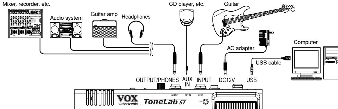
1. Set the AMP/LINE switch appropriately for the type of device you'll be connecting to the OUTPUT/PHONES jack. Set the AMP/LINE switch as follows.
