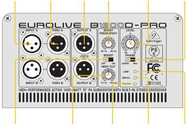
BOOST switch adds +6 dB of boost HIGH CUT controls upper corner frequency for subwoofer's amplifier. Does not affect THRU A/B or OUTPUT A/B signals
